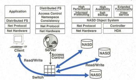
NASD's direct transfers between client and disk allow scalable bandwidth, lower latency, and off-load much of the file server's work without integrating file system policy into the disk.
