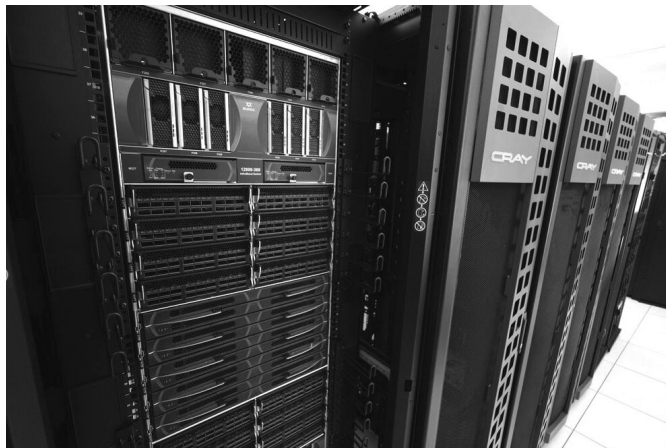
Wolf Cluster: QLogic 640-port InfiniBand Switch
