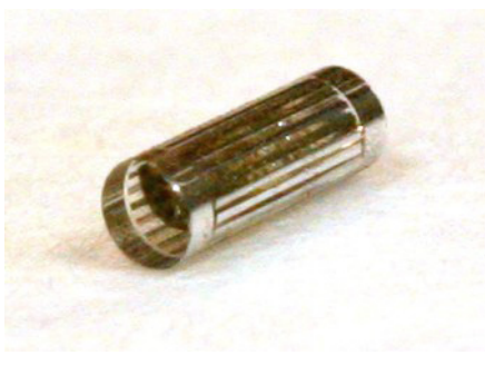
A prototype 1mm diameter tube housing a claytronics control-die.
