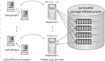
Figure 3. Head-end systems act as bridges into the storage infrastructure, translating NFS commands into the infrastructure's internal protocols.
