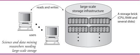
Figure 1. Brick Based infrastructure: a case study for understanding data center challenges and proving ground for new self-management approaches.
