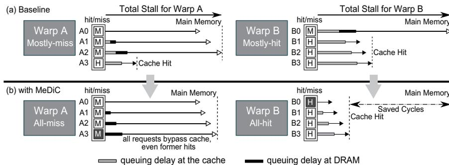
(a) Existing inter-warp heterogeneity, (b) exploiting the heterogeneity with MeDiC to improve performance.
