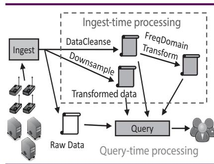
Ingest-time processing and query-time processing. Three transformation outputs are generated from the raw data. FreqDomainTransform is chained after DataCleanse.
