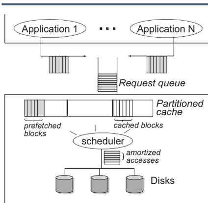
Argon's high-level architecture. Argon makes use of cache partitioning, request amortization, and quanta-based disk time scheduling.
