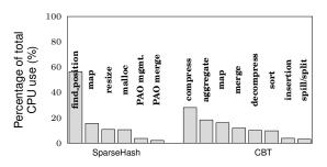
Figure 8: Comparison of CPU use by SparseHash (20 instances) and CBT (4 instances): For SparseHash, find\_position: find an unassigned index in a closed hashtable, map: map-side processing (tokenizing of keys etc.), resize: hashtable resizing when full, malloc: memory allocation, PAO mgmt.: creation of PAOs for insertion into hashtable, PAO merge: merging of PAOs with the same key. For CBT, each bar refers to the respective operation performed on buffer fragments in CBT nodes.
