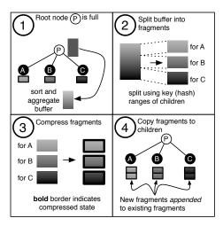
**Figure 3:** Spill process for root node *A*: The root buffer is sorted and aggregated; the buffer is then split into fragments according to hash ranges of children, and each fragment is compressed and copied into the respective children node.
