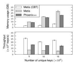
**Figure 9:** Comparison of CBT with aggregators in Metis and Phoenix++: All systems sort final results by count and display the top 5 words. The synthetic datasets consist of an increasing number of unique keys, with average key length 16B, and each key repeating 1000 times.
