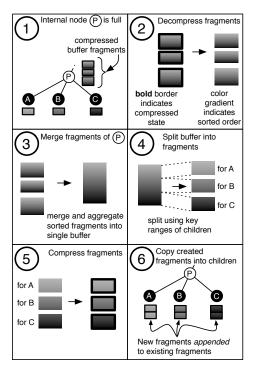
**Figure 5:** Spill process for internal node *P*: The compressed fragments in *A* are decompressed, merged (each is sorted), and split into fragments according to hash ranges of children. Each compressed fragment is copied into the respective child.
