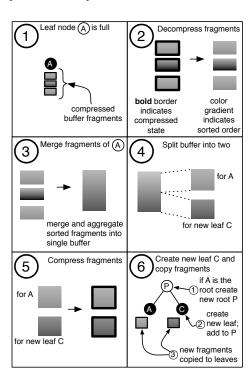
**Figure 4:** Split process for leaf node *A*: The compressed fragments in *A* are decompressed, merged (each is sorted), and divided into two splits. Both splits are compressed and one split copied into a new leaf node *C*.
