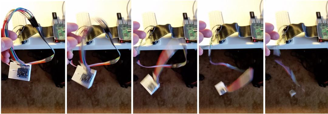
Figure 7.1. Snapshots of accelerometer being dropped from a height to simulate a fall.
