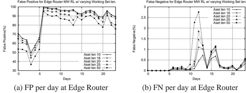
Figure 3: Results for Williamson's RL mechanism at Edge Router
