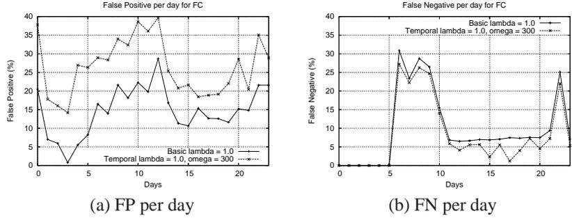
Figure 4: Error rates per day for Basic and Temporal FC with  $\lambda = 1.0$  &  $\Omega = 300$ .
