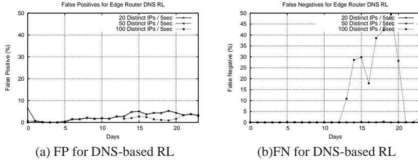
Figure 9: Results for DNS-based RL at the Edge Router
