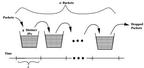
Figure 7: Cascading Bucket RL Scheme
