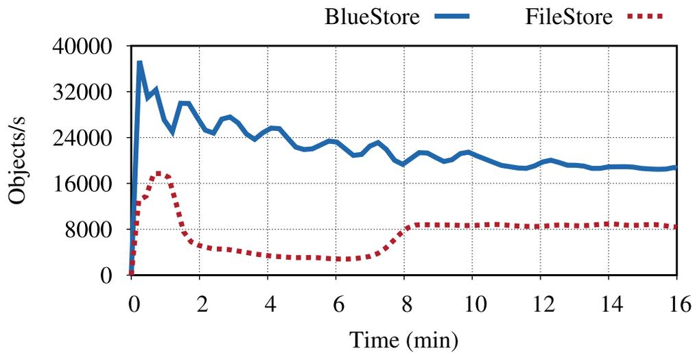
Fig. 10. Throughput of 4-KiB RADOS object writes with queue depth of 128 on a 16-node all-SSD cluster. At steady state, BlueStore is 2× faster than FileStore on SSD. BlueStore does not suffer from directory splitting; however, its throughput is gradually brought down by the RocksDB compaction overhead.
