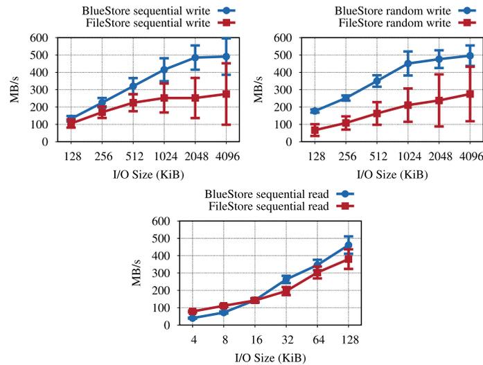
Fig. 11. Sequential write, random write, and sequential read throughput with different I/O sizes and queue depth of 256 on a 1 TB Ceph virtual block device (RBD) allocated on a 16-node all-HDD cluster. Results for an all-SSD cluster were similar but not shown for brevity.
