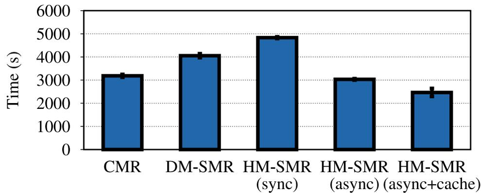
Fig. 13. Benchmark runtimes of the CMR and DM-SMR baselines and RocksDB on HM-SMR iterations. The benchmark performs 150 million *asynchronous* inserts of key-value pairs of size 20 bytes and 400 bytes, respectively.
