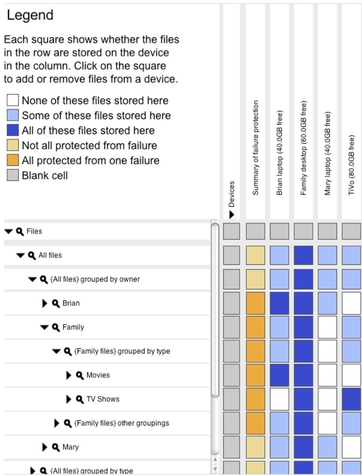
Figure 2: **View manager interface.** A screen shot of the view manager GUI. On the left are files, grouped using faceted metadata. Across the top are devices. Each square shows whether the files in the row are stored on the device in the column.
