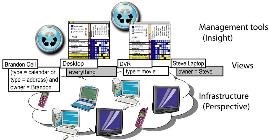
Figure 1: **View-based architecture.** Views are the interface between management tools and the underlying heterogeneous, disconnected infrastructure. By manipulating the views, tools can specify data policies that are then enforced by the filesystem.
