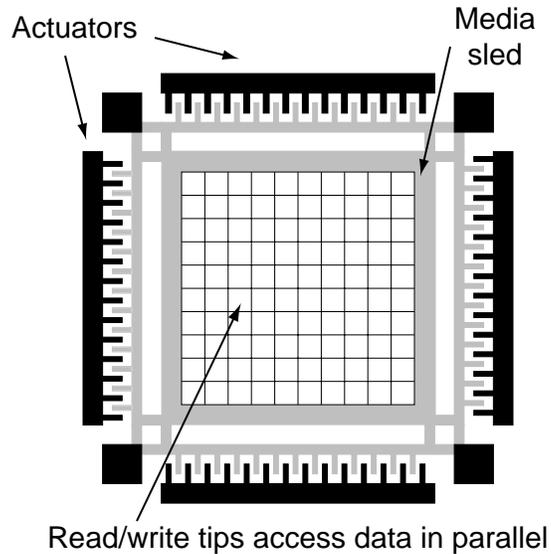
Figure 1: **High-level view of a MEMStore.** The major components of a MEMStore are the sled containing the recording media, MEMS actuators that position the media, and the read/write tips that access the media. The simplified device shown here has a ten by ten array of read/write tips, each of which accesses its own portion (or *square*) of the media. As the media is positioned, each tip accesses the same position within its square, thus providing parallel access to data.
