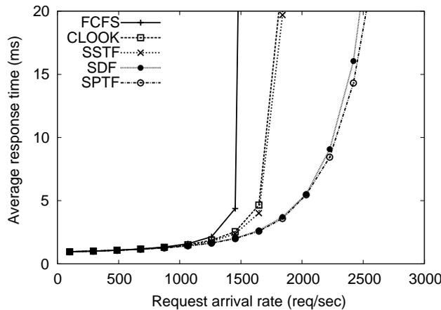
Figure 8: **Performance of shortest-distance-first scheduler without settle time.** If post-seek settle time is eliminated, then the seek time of a MEMStore becomes strongly correlated with both the X and Y positions. In this case, a scheduler that takes into account both dimensions provides a great deal better performance than those that only considers a single dimension (CLOOK and SSTF).
