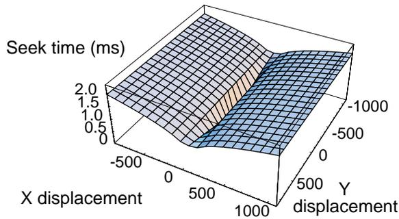
Figure 2: **MEMStore seek curve.** The seek time of a MEMStore is largely uncorrelated with the displacement in the Y dimension due to a large settling time applied to the X dimension seek time that is not applied to the Y dimension seek time [6, 10]. The overall seek time is the maximum of the two independent seek times.
