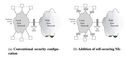
(a) shows the common network security configuration, wherein a firewall and a NIDS protect LAN systems from some WAN attacks. (b) shows the addition of self-securing NIs, one for each LAN system.
