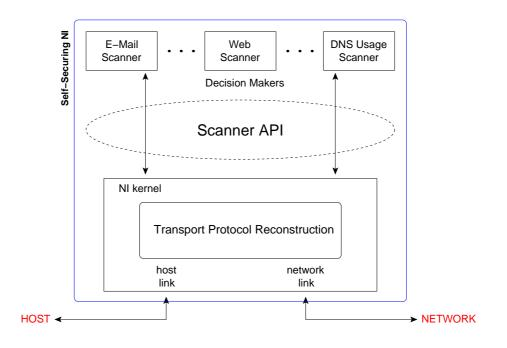
A "NI kernel" manages the host and network links. Scanners run as application processes. Scanner access to network traffic is limited to the API exported by the NI kernel.
