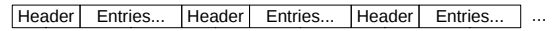
Figure 4: Pattern PLFS index file format. The headers indicate the type and size of the entries following them.
