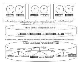
Figure 2: **PLFS Architecture.** This figure shows how PLFS maintains the user's logical view of a file which physically distributing it into many smaller files on an underlying parallel file system.
