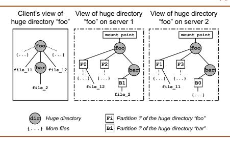
Local representation of huge directory in Giga+ prototype layered on Ext3 — Currently, we replicate the huge directory tree structure (not the files or partitions) for ease of namespace management through common path-name manipulation across all servers.
