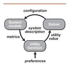
Overview of a utility-based provisioning tool. The solver produces candidate system configurations. The system models annotate the configurations with system, workload, and dataset metrics. The utility function uses the administrator's preferences to rank the annotated configurations by assigning a utility value to each.
