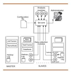
Deploying ASDF and its modules for a Hadoop cluster. The fpt-core runs on the ASDF control node. performance problems in Hadoop, under different workloads; our results indicate that ASDF incurs an average monitoring overhead of 0.38% of CPU time, and exhibits average online fingerpointing latencies of less than I minute with false-positive rates of less than I%.
