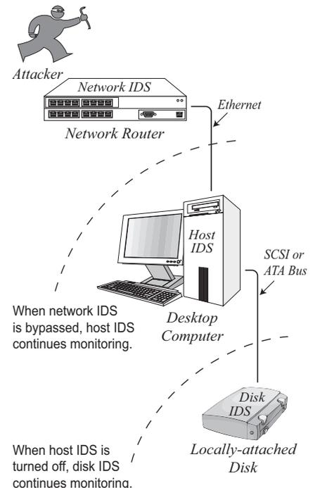
The role of a disk-based intrusion detection system (IDS). A disk-based IDS watches over all data and executable files that are persistently written to local storage, monitoring for suspicious activity that might indicate an intrusion on the host computer.
