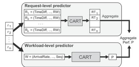
Per-request and feature-based predictors.  $r_i$  is the  $i$ -th request in the workload;  $RT_i$  is the response time of  $r_i$ ;  $R_i$  is the set of per-request characteristics for  $r_i$ ;  $W$  is the set of workload-level characteristics.
