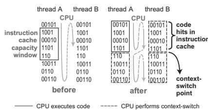
**Before:** As the instruction cache cannot fit the entire code, when the CPU switches (dotted line) to thread B it will incur the same number of misses. **After:** If we “break” the code into several pieces that fit in the cache, and switch execution back and forth between the two threads, thread B will find all instructions in the cache.
