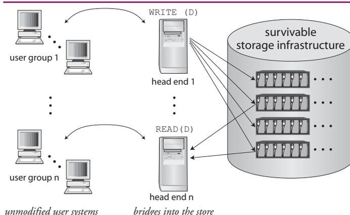
Figure 3. Head-end systems act as bridges into the storage infrastructure, translating NFS commands into the infrastructure's internal protocols.
