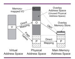
Overview of our design. "Direct mapping" indicates that the corresponding mapping is implicit in the source address. OMT = Overlay Mapping Table
