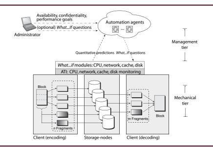
**High-level architecture of Ursa Minor.** The mechanical tier, on the bottom, services I/O requests for clients. The management tier, on the top, provides automation. It makes use of the self-predicting capabilities of the individual system components to get answers to various *What...if* explorations.
