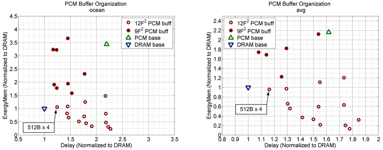
**Figure 5: Pareto analysis for ocean (L) and benchmark average (R). Open circles indicate designs satisfying area constraints assuming  $12F^2$  PCM multi-level cells. Closed circles indicate additional designs satisfying area constraints assuming smaller  $9F^2$  PCM multi-level cells.**
