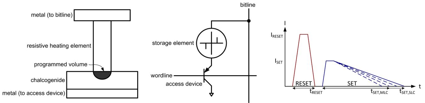
**Figure 1: Phase Change Memory.** Storage element with heating resistor and chalcogenide between electrodes (L). Cell structure with storage element and BJT access device (C). RESET to an amorphous (high resistance) state with a high, short current pulse. SET to a crystalline (low resistance) state with moderate, long current pulse. Slope of SET current ramp down determines the state in multi-level cells (R).
