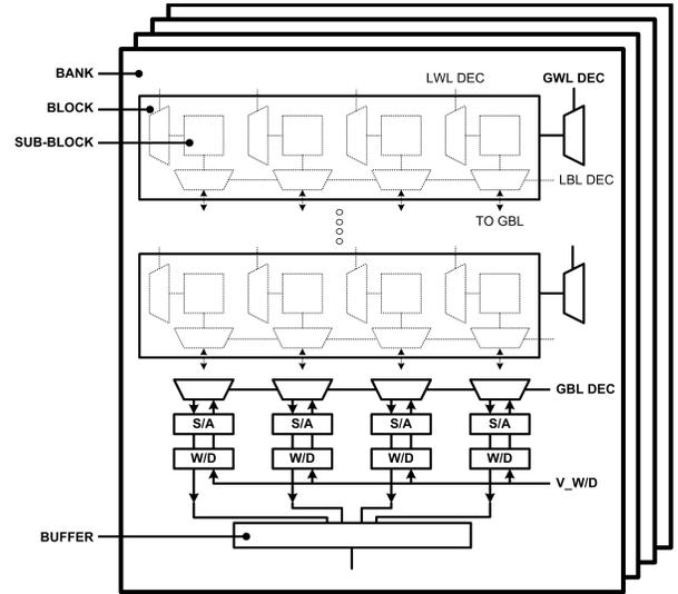
**Figure 3: Array Architecture.** A hierarchical memory organization includes banks, blocks, and sub-blocks with local, global decoding for row, column addresses. Sense amplifiers (S/A’s) and word drivers (W/D’s) are multiplexed across blocks.
