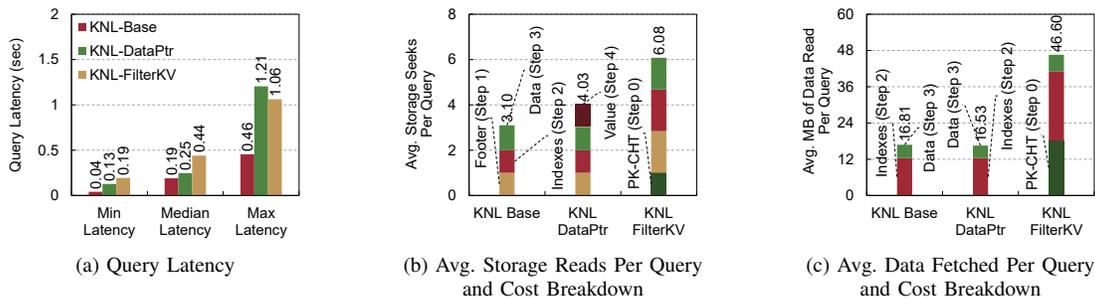
Fig. 11: Performance of reading individual particles from a 2TB dataset. FilterKV shows comparable latency with the base format and the current state-of-the-art. In (b) and (c), cost is categorized by the type of data read from storage. PK-CHT stands for partial-key cuckoo hash tables.
