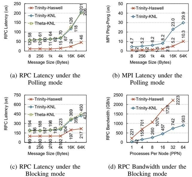
Fig. 1: Results from LANL (Trinity) and ANL (Theta) comparing RPC performance between an Intel multicore processor (Haswell) and two Intel manycore processors (KNL). For reference, we also show in Figure (b) MPI ping-pong latency numbers obtained using the OSU benchmark.
