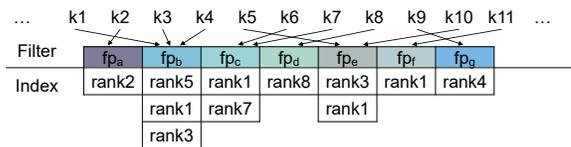
Fig. 5: A hybrid auxiliary table design using both filters and indexes. Keys are stored as small fingerprints in a filter. Each fingerprint is mapped to one or more ranks at the index layer. False positives are still possible because multiple keys may be mapped to a single key fingerprint. Readers nevertheless can quickly retrieve the ranks mapped to a key using a single filter and index lookup; no exhaustive filter tests are needed.
