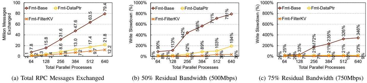
Fig. 8: Results comparing the performance of different online data partitioning schemes under different job sizes. We vary job size from 64 (16 nodes) to 640 parallel processes (160 nodes). Each run generates 15 million KV pairs per process. Each KV pair is 64 bytes.
