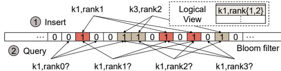
Fig. 4: Compactly mapping keys to ranks using Bloom filters. Step 1 inserts two key-rank mappings into the filter, turning two subsets of the filter’s bits from 0 to 1. Step 2 retrieves  $k1$ ’s mapping by exhaustively checking all possible mappings for  $k1$ . Due to false positives, a Bloom filter may map a key to one or more ranks. In this example, there are 4 ranks and  $k1$  is mapped to both rank 1 (True positive) and 2 (False).
