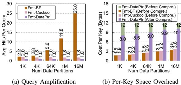
Fig. 7: Comparison of three different data partitioning schemes. Fmt-DataPtr is the current state-of-the-art. Figure (b) shows Fmt-DataPtr’s space usage both before and after data compression is applied.
