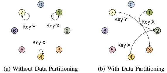
Fig. 2: **Distributed processes of a parallel application writing data output.** Without data partitioning, data is streamed to per-process files so per-key data ends up in multiple files and reading a key may require searching all files. With data partitioning, each key is sent to a particular process so that reading a key requires searching only a single data partition.
