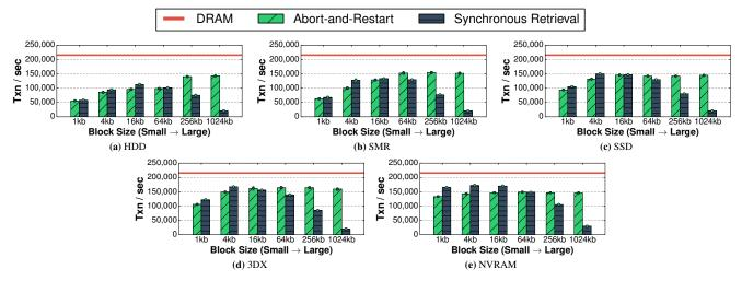
Figure 2: Cold Tuple Retrieval – Throughput for the YCSB workload in H-Store with anti-caching when using different storage devices with the two retrieval policies from Sect. 4.1. For each device and retrieval configuration, we scale up the size of the cold tuple blocks from 1 to 1024 KB.
