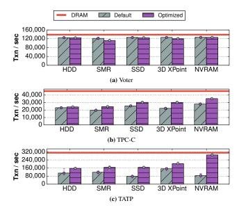
**Figure 6:** Additional Workloads – Throughput measurements for H-Store with anti-caching when using the optimal hardware-dependent policy configuration for each storage device compared to a default configuration.
