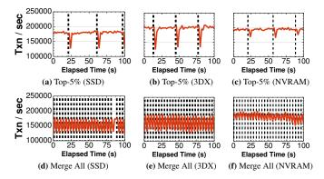
**Figure 4: Merging Threshold (Sustained Throughput)** – Throughput for YCSB in H-Store under different merge threshold policies. The vertical bars denote when the DBMS evicts tuples out to secondary storage. The y-axis represents the real-time throughput of the DBMS in every second.
