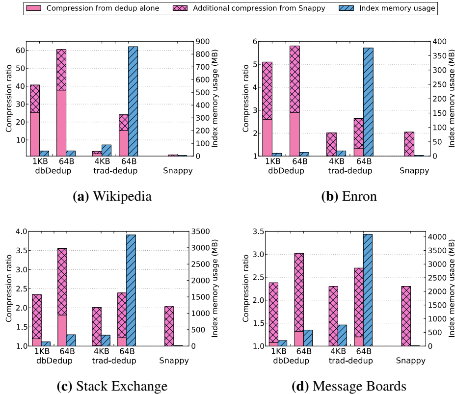
Figure 6.1: Compression Ratio and Index Memory – The compression ratio and index memory usage for dbDedup (1 KB chunks or 64 byte chunks), trad-dedup (4 KB and 64 byte), and Snappy. The upper portion of each dedup bar represents the added benefit of compressing after dedup.
