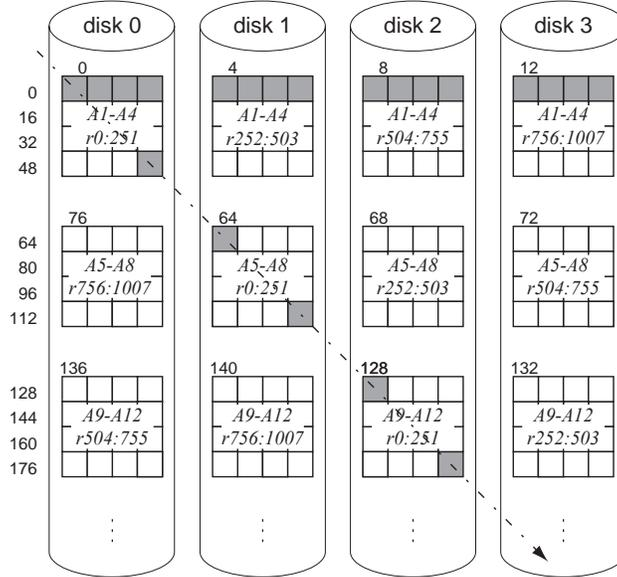
Figure 5: Mapping of a database table with 12 attributes onto *Atropos* logical volume with 4 disks. The numbers to the left of disk 0 are the *LBNs* mapped to the gray disk locations connected by the arrow and not the first block of each row. The arrow illustrates efficient semi-sequential access fetching single A-page with 63 records. A single sequential I/O for 16 *LBNs* can efficiently fetch one attribute from 1008 records striped across four disks.
