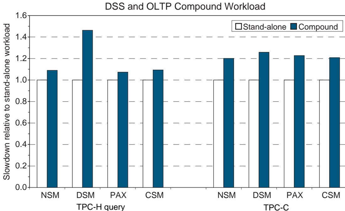
Figure 10: **Compound workload performance for different layouts.** This figure shows the slowdown off TPC-H query 1 runtime when run with TPC-C benchmark relative to the case when runs in isolation and the impact on TPC-C performance.
