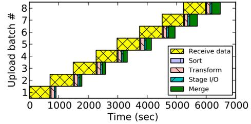
**Figure 8.** Ingest pipeline profiling for the occurrence count use case. This figure shows the amount of time that each upload batch spends at each pipeline stage, when we generate six count-min-sketch transformations.
