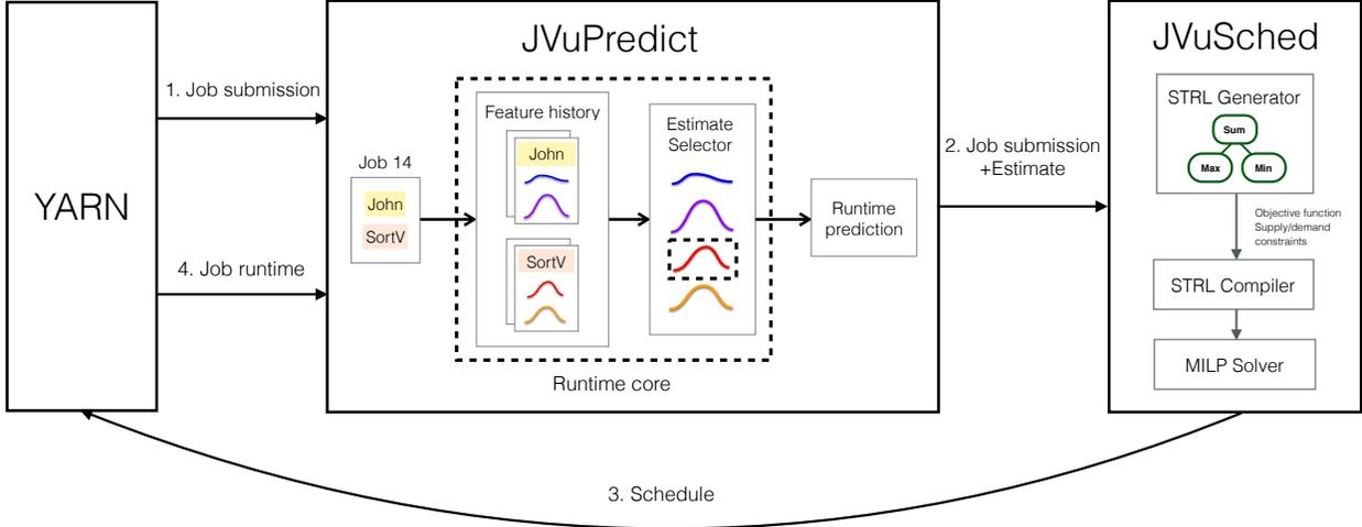
Figure 7: End-to-end system integration
