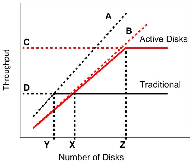
To the left of point Y, the traditional system is disk-bound. Below the crossover point X, the Active Disk system is slower than the server system due to its less powerful CPU. Above point Z, even the Active Disk system is network-bottlenecked and no further improvement is possible.
