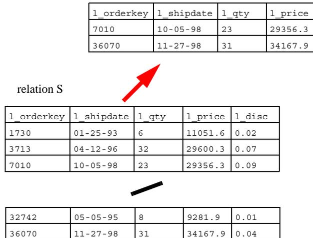
Figure 4-6 Illustration of basic select operation in a database system. A single relation is searched for attributes that match the given value. Note that there are two types of data reduction going on here. The first is the selection of matching records (5% in this example from TPC-D) and the second is the elimination of unneeded columns from the relation (3/4 of the data in this example).
