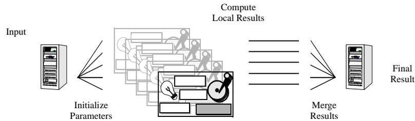
Figure 6-1 Basic structure of Active Disk computation. The host initializes the computation, each of the drives computes results for its local data, and these results are combined by the host.
