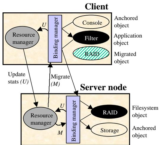
Figure 2: The architecture of the ABACUS migration system. An application is broken up into a number of migratable objects. Calls between the objects are redirected by binding managers that know where the objects are currently running. Binding managers also inform resource managers about the resources consumed by the objects. The resource managers use this information to reevaluate how objects are partitioned among clients and servers.
