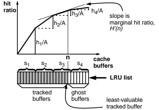
**Figure 9. Piecewise estimation of  $H(n)$ .** The LRU list is broken into segments,  $s_1, s_2, s_3, \dots$ . Each buffer is tagged to indicate which segment it is in. The tag is updated when a buffer passes from one segment to the next. When there is a cache hit in segment  $i$ , the segment hit count,  $h_i$ , is incremented. That segment's contribution to the hit ratio is then  $h_i/A$ , where  $A$  is the total number of accesses to the LRU cache.
