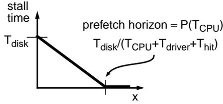
**Figure 4. Worst case stall time and the prefetch horizon.** Data consumption is limited by the time an application spends acquiring and consuming each block. This graph shows the worst case application stall time for a single prefetch  $x$  accesses in advance, assuming adequate I/O bandwidth, and therefore no disk queues. There is no benefit from prefetching further ahead than the prefetch horizon.
