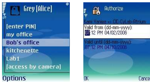
Figure 1: Left: Main screen containing all the resources the phone knows about, clicking on a resource causes the phone to attempt to unlock it. Right: A user proactively creating a delegation.
