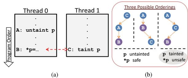
Figure 1: Impact of inter-thread data dependences on TAINTCHECK. Instruction A (C) untaints (respectively, taints) *p*. (a) The safety of *\*p* in instruction B depends on (b) which of the interleavings occur.
