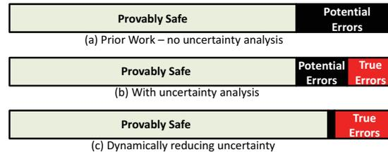
Figure 2: Dividing memory operations into provably safe (precise), true error (precise) and potential errors (conservative). Tracking uncertainty enables separation of potential errors and true errors; dynamic adaptations reduce analysis uncertainty.
