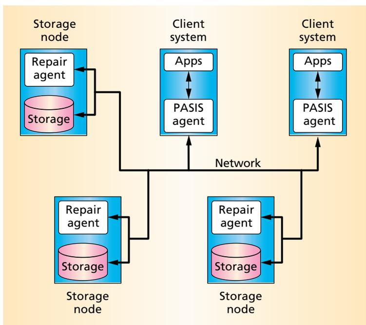
**Figure 1.** The PASIS architecture. Client systems and storage nodes are attached to the network. Client applications interact with a PASIS storage system through a PASIS agent. Storage devices and repair agents that monitor system status comprise the storage nodes.
