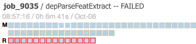
Figure 3: Visual signature of bugs in the Reduce phase. Failures spread across all Reduce nodes (solid dark/red border) typically signal a bug in the Reduce phase.
