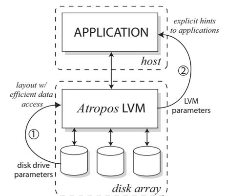
**Atropos logical volume manager architecture.** Atropos exploits disk characteristics (arrow 1), automatically extracted from disk drives, to construct a new data organization. It exposes high-level parameters that allow applications to directly take advantage of this data organization for efficient access to one- or two-dimensional data structures (arrow 2).
