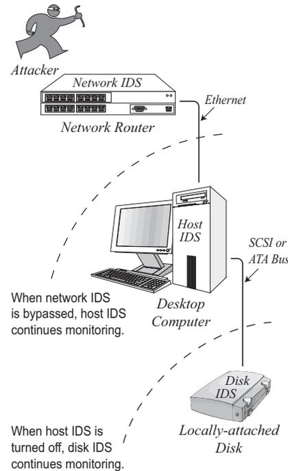
**The role of a disk-based intrusion detection system (IDS).** A disk-based IDS watches over all data and executable files that are persistently written to local storage, monitoring for suspicious activity that might indicate an intrusion on the host computer.
