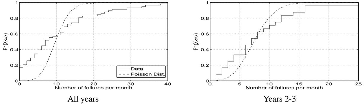
Figure 5: *CDF of number of failures per month in HPC1*
