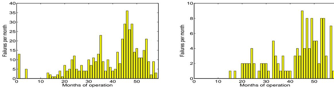
Figure 4: Number of failures observed per month over the first 5 years of system HPC1’s lifetime, for the compute nodes (left) and the file system nodes (right).
