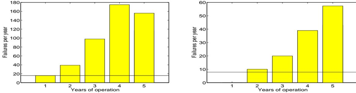
Figure 3: Number of failures observed per year over the first 5 years of system HPC1’s lifetime, for the compute nodes (left) and the file system nodes (right).
