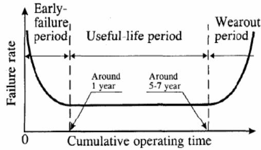
Figure 2: *Life cycle failure pattern of hard drives [27].*
