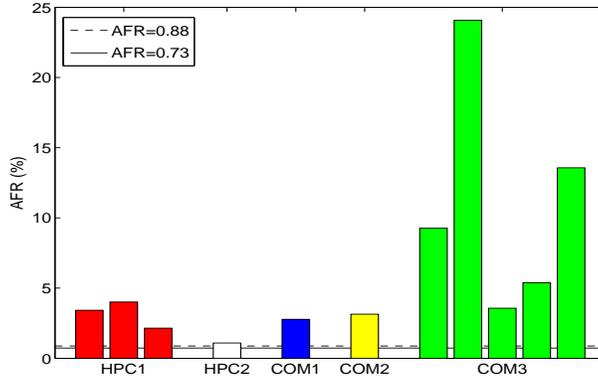
Figure 1: Comparison of datasheet AFRs (solid and dashed line in the graph) and AFRs observed in the field (bars in the graph). Left-most bar in a set is the result of combining all types of disks in the data set.
