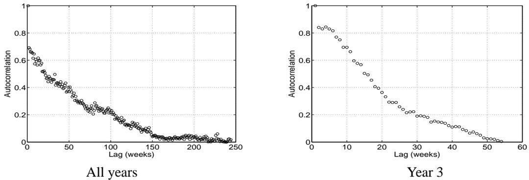
Figure 7: *Autocorrelation function for the number of failures per week computed across the entire lifetime of the HPC1 system (left) and computed across only one year of HPC1’s operation (right).*
