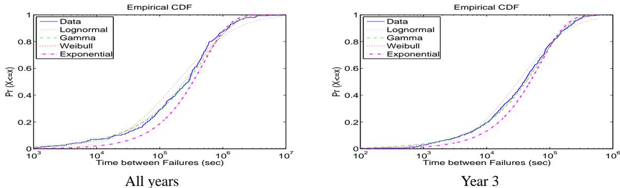
Figure 8: *Distribution of time between failures across all nodes in HPC1.*
