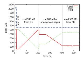
**6: Unified buffer cache.** This figures shows the amount of memory consumed by the user and FSVA VMs. As applications shift their memory access pattern between file system and virtual memory usage, the unified buffer cache dynamically allocates memory among the two VMs while maintaining a constant total memory allocation.
