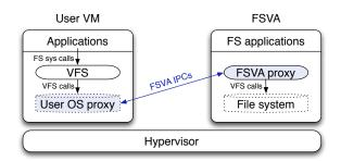
**2:** FSVA architecture. An FS and its (optional) management applications run in a dedicated VM. An FS-agnostic proxy running in the client OS and FSVA pass VFS calls via an efficient IPC transport.
