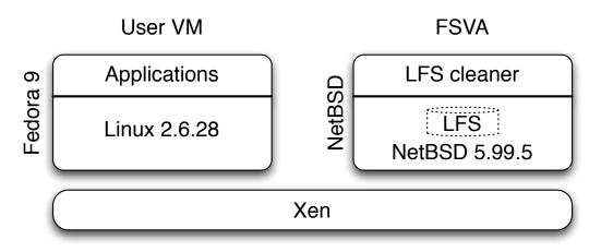
1: A file system runs in a separate VM. A user continues to run their preferred OS. By decoupling the user and FS OSs, one allows users to use any OS without needing a corresponding FS port. As an example, Linux does not include a log-structured file system (LFS) implementation. But, using FSVAs, a Linux user can utilize NetBSD's LFS implementation. This illustrated example is used as a case study in §5.2.
