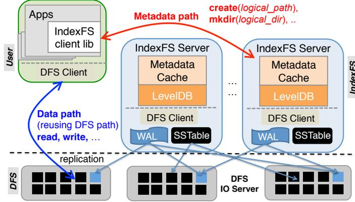
Figure 1: The IndexFS metadata system is middleware layered on top of an existing cluster file system deployment (such as PVFS) to improve metadata and small file operation efficiency. It reuses the data path of the underlying file system and packs directory entries, file attributes and small file data into large immutable files that are stored in the underlying file system.
