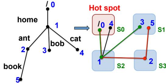
Figure 2: The figure shows how IndexFS distributes a file system directory tree evenly into four metadata servers. Path traversal makes some directories (e.g. root directory) more frequently accessed than others. Thus state-less directory caching is used to mitigate these hot spots.
