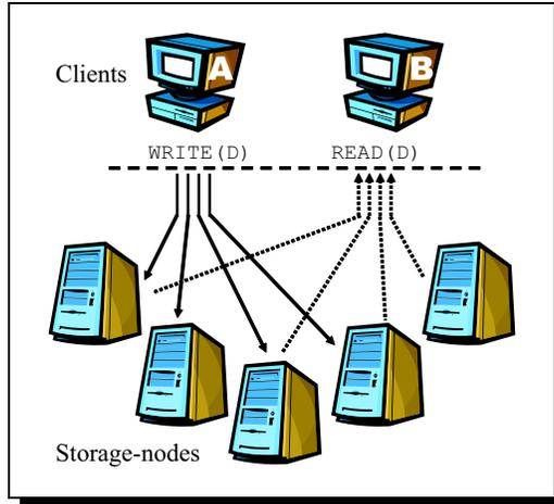
Figure 1: **High-level architecture for survivable storage.** Spreading data redundantly across storage-nodes improves its fault-tolerance. Clients write and (usually) read data from multiple storage-nodes.
